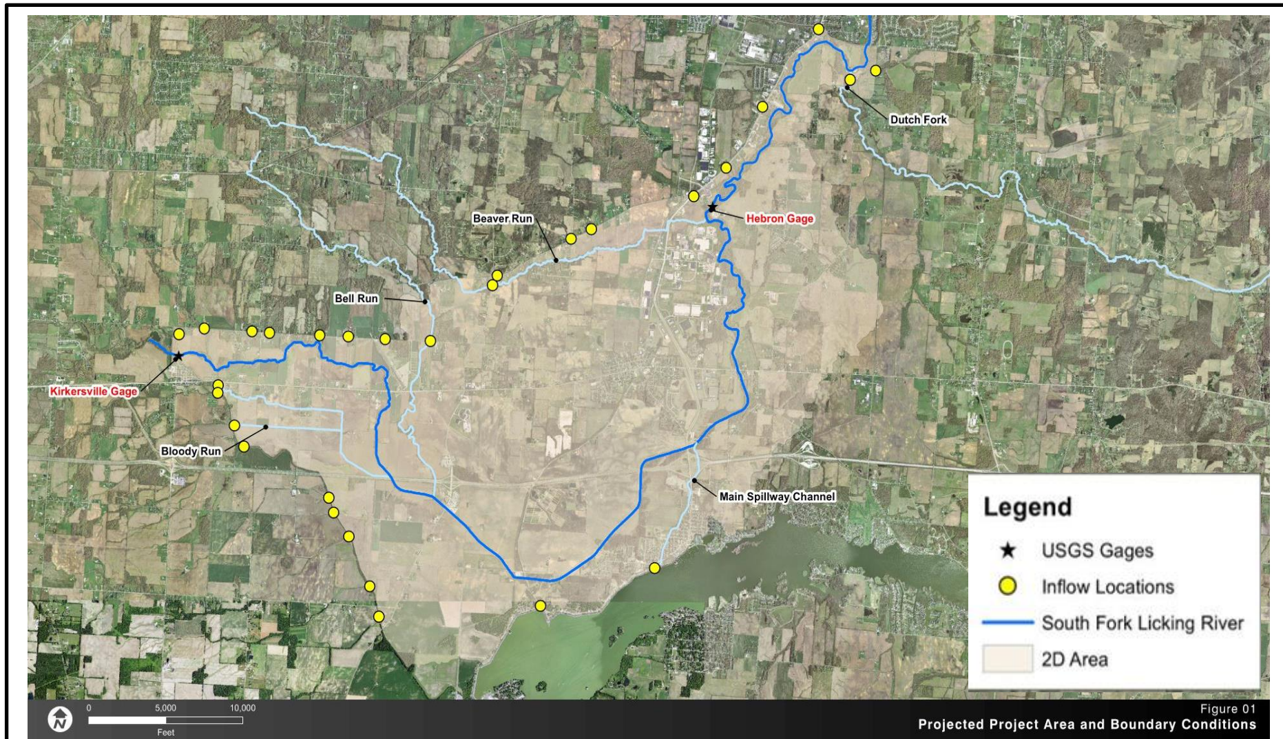
FIGURE 6-3 Watershed Interface Points between HEC-HMS and 2D HEC-RAS Models (Image prepared by ms consultants)
